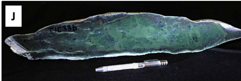
H-K) Representative polished samples of Nephrite Jade from Trench T1C, showing range of textures and colors. H) Sample T1C36b, 13 pounds (5.9 Kg), 33.5 by 11.5 centimeters. I) Sample T1C22b, 6 pounds (2.7 Kg), 36x8.5 cm. J) Sample T1C33b, 6 pounds (2.7 Kg), 43x11.5 cm and K) Sample T1C32b, 15 pounds (6.8 Kg), 56.5x13.5 centimeters. Mounted on a cedar base to show the Jade's color and texture.
